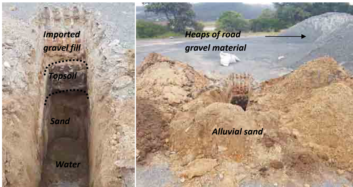
Figure 6: Typical test pit showing water table and soil types (TP5)
