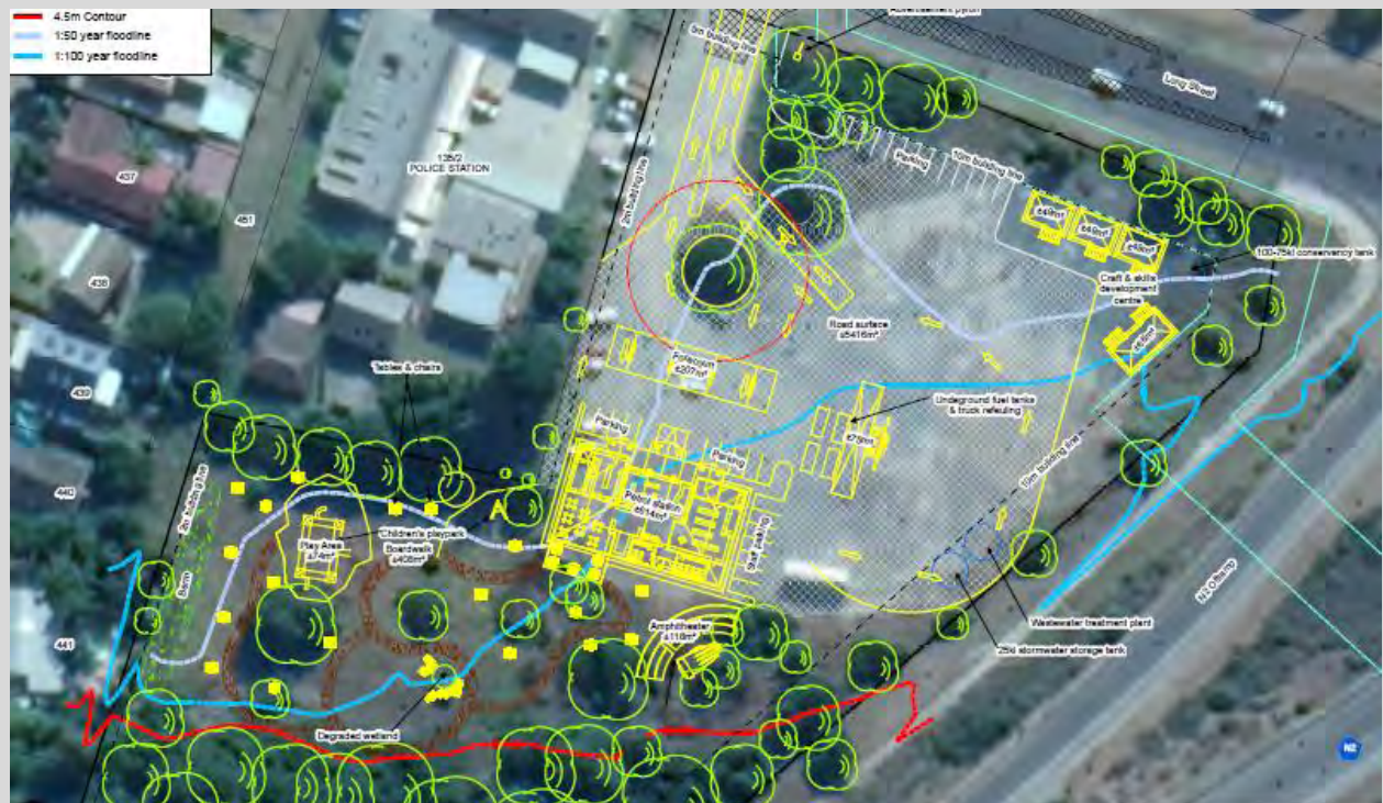
Figure 7: Preferred Alternative 1 Layout in relation to 1:50 & 1:100 year floodlines of estuary & 4.5m contour line.
