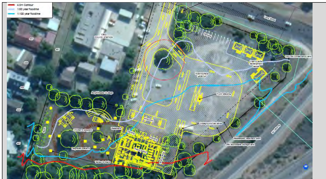
Figure 8: Alternative 2 layout in relation to 1:50 & 1:100 year floodlines of estuary & 4.5m contour line.
